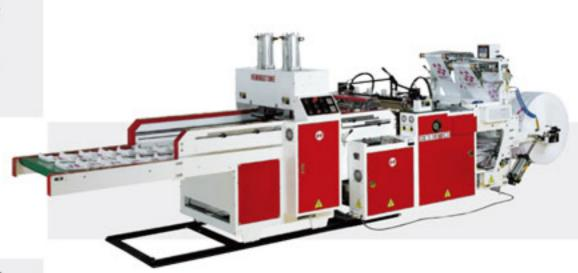
High Speed 2 Lines Fully Automatic T-Shirt Bag Making Machine with Servo-Drive System for Japan Market (400 PCS/MIN) HM-800JT (Non Stop)
