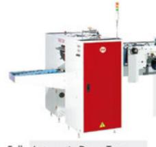
Fully Automatic Draw Tape Garbage Bag Making Machine for Overlap & Perforation Bag-on-Roll (120 PCS/MIN) (Non Stop)
