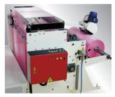
• This machine can simultaneously produce bottom sealing bags
